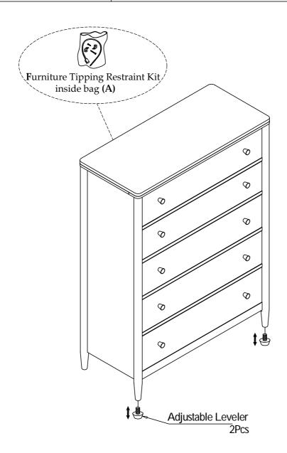
For product and personal safety, a Furniture Tipping Restraint kit has been included with this unit which can help to minimize the risk of the unit accidentally tipping forward, if used and properly installed per the kit manufacturer's instructions.
